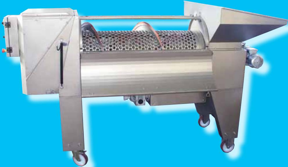
adjust the speed of the load. A filter is installed for the extraction of the liquid and a fitting for connection of an external pump. The screw is made with a circular profile rounded.
