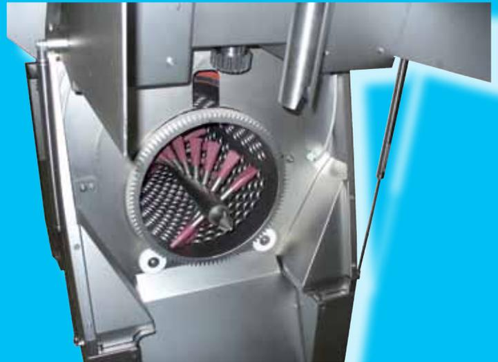
The speed of the basket and the shaft is handled through an electronic speed control with digital display: the immediate selection of the speed allows the user to optimize the destemming.
